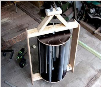
Vertical axis wind turbine from Windsol Power, the runner-up project
